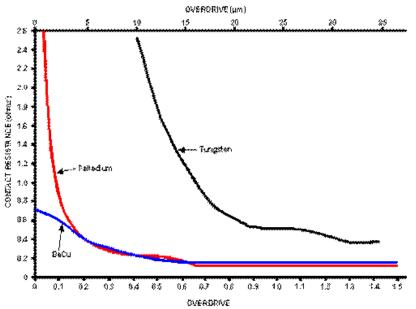
Accuprobe does not offer a Palladium alloy tip because of the difficulty maintaining planarity with this material. There is clearly a relationship of contact resistance to overdrive as discussed earlier,
